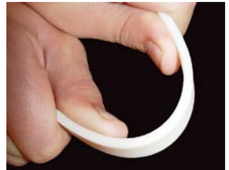
Accura ® 25 Plastic has high flexibility, while retaining the original shape.
